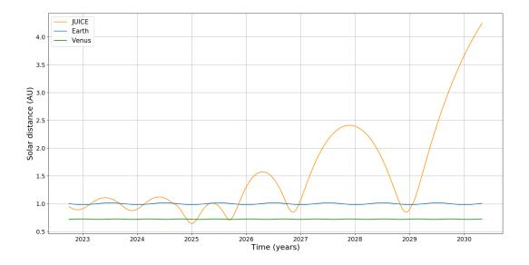
Figure 3.3: Solar distances of JUICE, Venus, and the Earth. The flybys are visible as crossing points.
