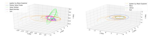
Figure 3.1: Left: The trajectories of JUICE and the other spacecraft. Right: The orbits of JUICE, Venus, and Mars.
