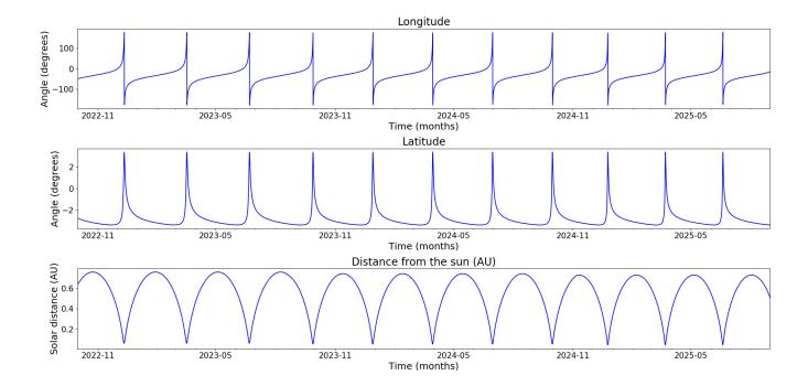
Figure 5.2: Coordinates of the Parker Solar Probe.
