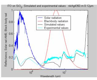
Fig. 4-20. Simulated and measured reflectance of ITO (type 4350) onto Corning 7059 glass.
