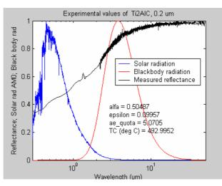
Fig. 4-15. Measured reflectance of thin film  $Ti_2AlC$ , 0.2 µm thick. The balance temperature was 490 °C and alfa/epsilon = 5.1.
