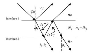
Fig. 2-1 Multiple reflections in a thin film layer of refractive index N1, the angle of incidence is  $\varphi 0$ , the substrate refractive index is n2 and the refractive index of the ambient medium is n0
