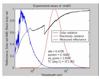
Fig. 4-6 Measured reflectance of nitrided TiAl, 0.2  $\mu$ m thick. The balance temperature was 370 °C and alfa/epsilon = 2.6.
