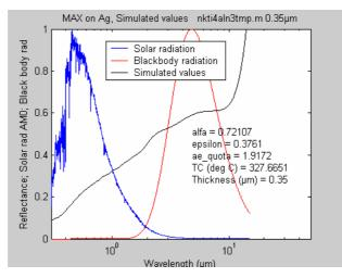
Fig. 4-10. Simulated reflectance of  $Ti_4AlN_3$  (on Ag) at a thickness of 0.35  $\mu$ m, yielding a balance temperature of 330 °C and alfa/epsilon = 1.9.
