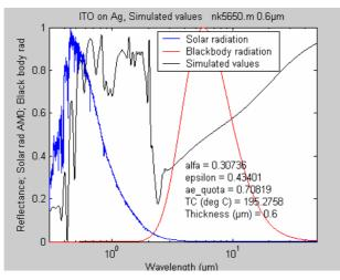
Fig. 4-19. Simulated reflectance of 0.6  $\mu$ m ITO (type 5650) on an Ag substrate. The balance temperature was 200 °C and alfa/epsilon = 0.71.
