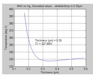
Fig. 4-9. Iteration of calculation of balance temperature for different thickness of  $Ti_4AlN_3$  (on Ag). The lowest temperature was 330 °C for 0.35  $\mu$ m.
