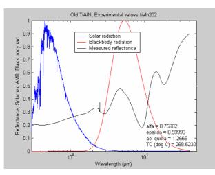
Fig. 4-1 Measured reflectance of previously sputtered TiAlN, 0.65  $\mu m$  thick. The balance temperature was 270 °C.
