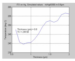
Fig. 4-24. Iteration of balance temperature calculations for different thickness of ITO (type 43300) on an Ag substrate. The lowest temperature was 240 °C for 0.8  $\mu$ m
