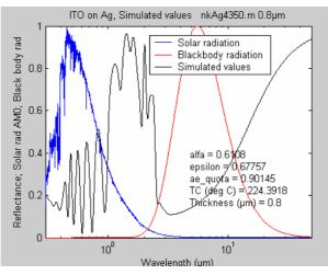
Fig. 4-22. Simulated reflectance of 0.8  $\mu$ m ITO (type 4350) on an Ag substrate. The balance temperature was 220 °C and alfa/epsilon = 0.9.
