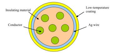
Fig. 1-1. Schematic cross-section of a co-axial boom cable with a low-temperature coating.
