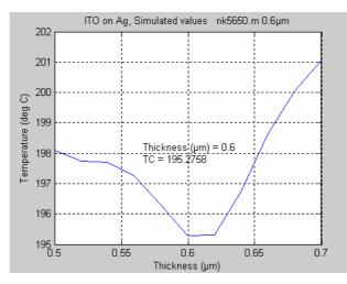
Fig. 4-18. Iteration of balance temperature calculations for different thickness of ITO (type 5650) on an Ag substrate. The lowest temperature was 200  $^{\circ}$ C for 0.6  $\mu$ m.
