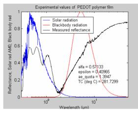
Fig. 4-26. Measured reflectance of a PEDT polymer onto Ag. The balance temperature was 280  $^{\circ}$ C and alfa/epsilon = 1.4.
