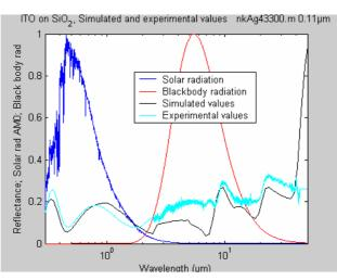
Fig. 4-23. Simulated and measured reflectance of ITO (type 43300) onto Corning 7059 glass.
