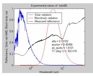
Fig. 4-3. Measured reflectance of sputtered TiAlN, 0.6  $\mu$ m thick. The balance temperature was 300 °C and alfa/epsilon = 1.6.
