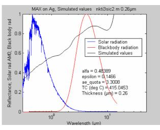
Fig. 4-12. Simulated reflectance of  $Ti_3SiC_2$  (on Ag) at a thickness of 0.26  $\mu$ m, yielding a balance temperature of 420 °C and alfa/epsilon = 3.3.
