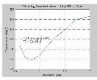
Fig. 4-21. Iteration of balance temperature calculations for different thickness of ITO (type 4350) on an Ag substrate. The lowest temperature was 220  $^{\circ}$ C for 0.8  $\mu$ m.
