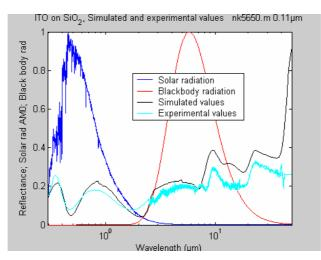
Fig. 4-17. Simulated and measured reflectance of ITO (type 5650) onto Corning 7059 glass.
