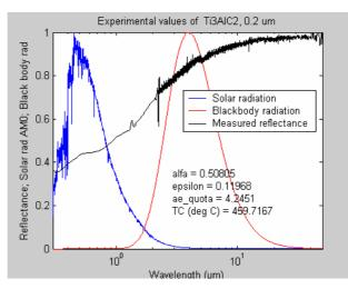
Fig. 4-13. Measured reflectance of thin film  $Ti_3AlC_2$ , 0.2 µm thick. The balance temperature was 460 °C and alfa/epsilon = 4.2.
