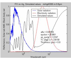
Fig. 4-25. . Simulated reflectance of 0.8  $\mu$ m ITO (type 43300) on an Ag substrate. The balance temperature was 240 °C and alfa/epsilon = 1.0.
