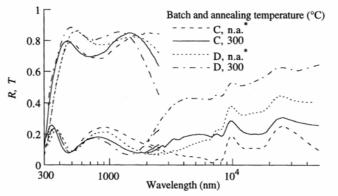
Figure 32: Spectral reflectance (R) and transmittance (T) for pure ITO samples from batches C and D, all deposited at room temperature and two were annealed at 300°C ( $T_A$ ). \* n.a. means no annealing. Tab. 5.25
