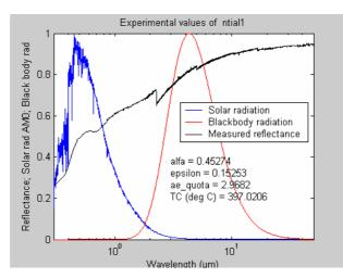
Fig. 4-8. Measured reflectance of nitrided TiAl, 1.0  $\mu$ m thick. The balance temperature was 400 °C and alfa/epsilon = 3.0.
