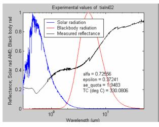
Fig. 4-2. Measured reflectance of sputtered TiAlN, 0.2  $\mu$ m thick. The balance temperature was 330 °C and alfa/epsilon = 1.9.
