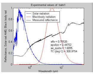
Fig. 4-4. Measured reflectance of sputtered TiAlN, 1.0  $\mu$ m thick. The balance temperature was 310 °C and alfa/epsilon = 1.7.
