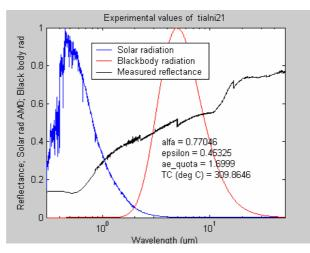
Fig. 4-5. Measured reflectance of sputtered TiAlN, 2.1  $\mu$ m thick. The balance temperature was 310 °C and alfa/epsilon = 1.7.
