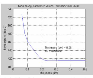
Fig. 4-11. Iteration of calculation of balance temperature for different thickness of  $Ti_3SiC_2$  (on Ag). The lowest temperature was 420 °C for 0.26  $\mu$ m.
