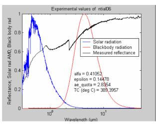
Fig. 4-7. Measured reflectance of nitrided TiAl, 0.6  $\mu$ m thick. The balance temperature was 390 °C and alfa/epsilon = 2.8.
