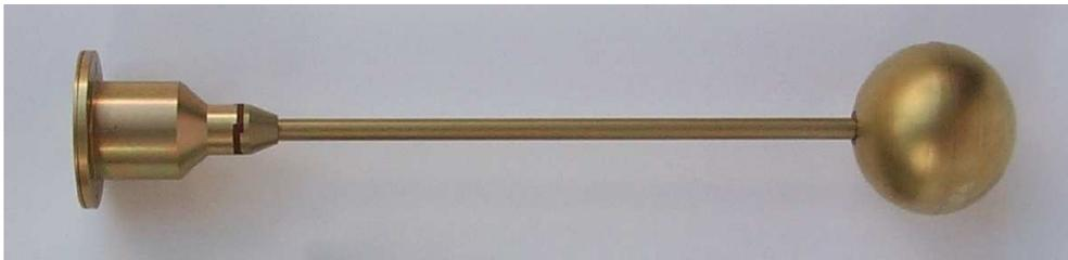
Figure 3: Rosetta Langmuir Probe.
