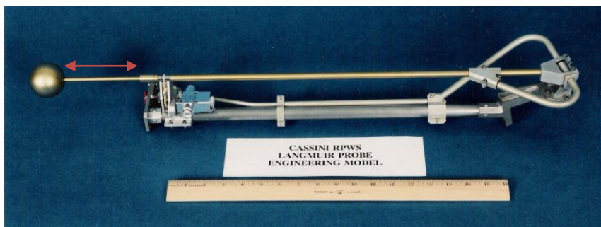
Figure 7. RWPS/LP, engineering model. The red arrow marks the stub that has same potential as the probe.
